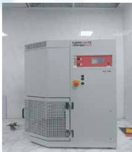
Glass Melting Furnace (1800 °C)
